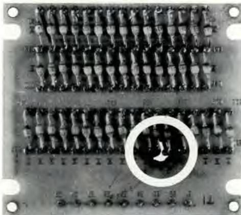
The silicate ester coolant was reacting with moisture to form a silica gel and alcohol. This gel buildup on electrical boards was causing system failures through electrical arcing.
