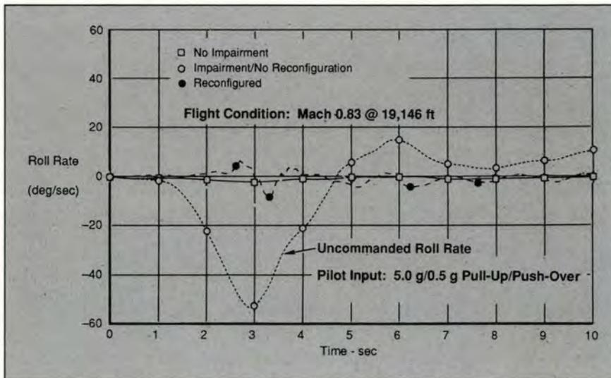
Figure 7. F-15 Flight Response Comparison: Pilot Commands a 5-g Pitch Maneuver With Right Stabilator Failed in Locked Position
