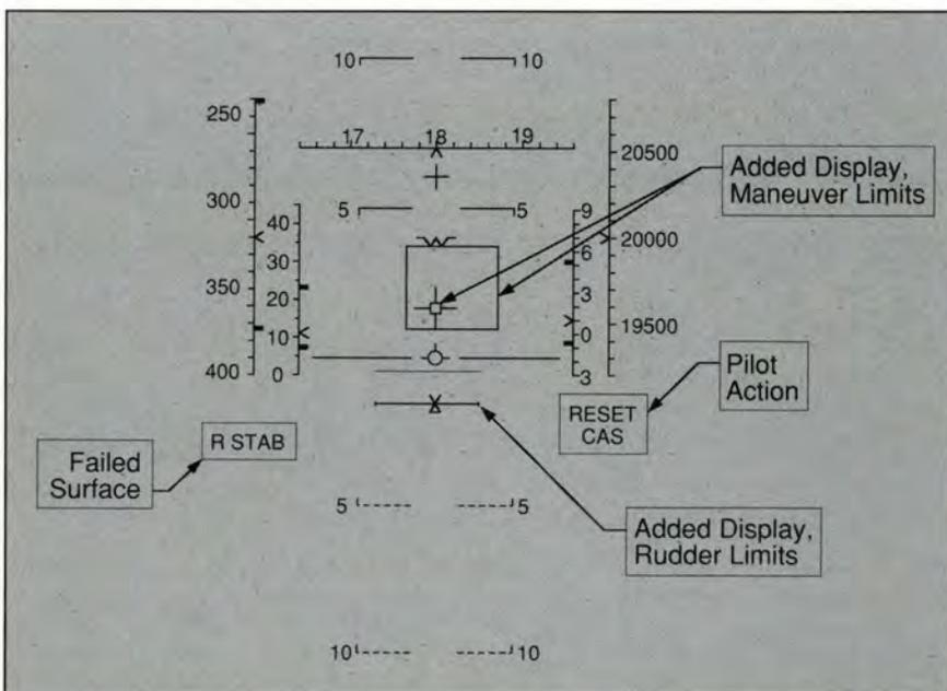
Figure 8. The HUD Shows Maneuver Capability of Damaged F-15
