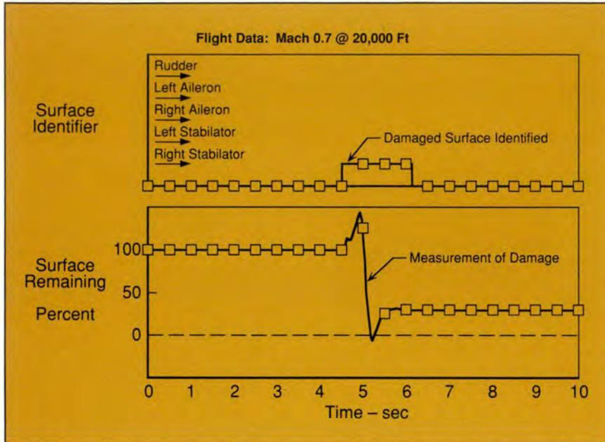
Figure 5. Flight Recording of Damage Detection, Right Stabilator of the Test F-15 Missing 80% of the Span Surface
