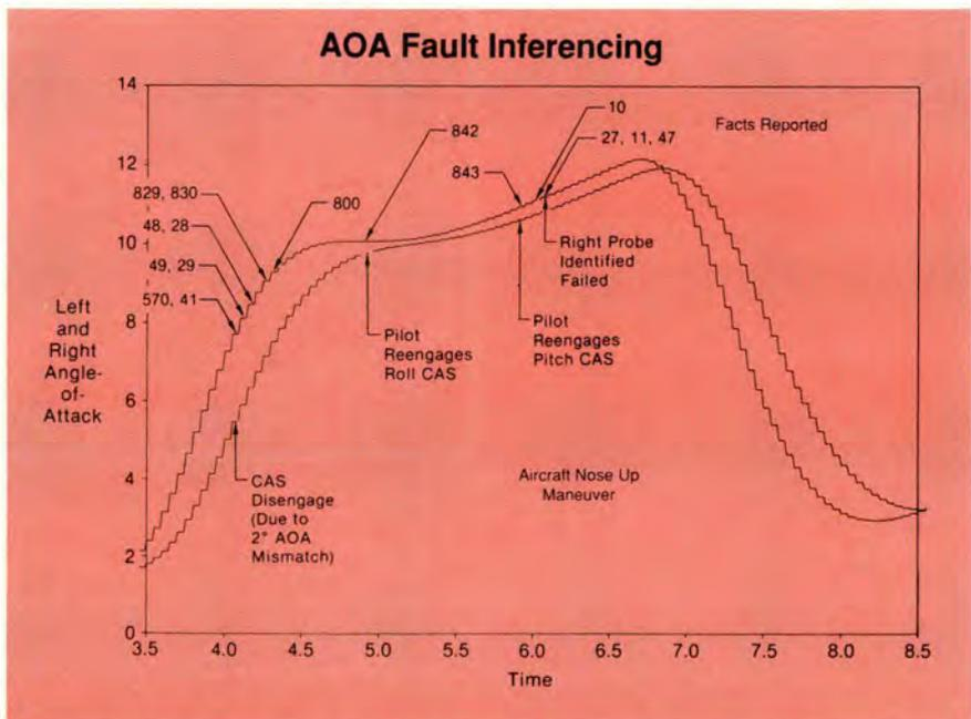
Figure 4. Flight Response With Fault Diagnostics Reporting Failure in F-15 Angle-of-Attack Sensor, Right Side
