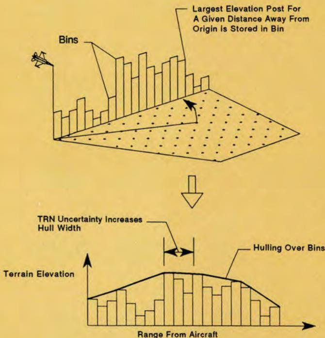
Figure 2 Binning and Hulling Process
