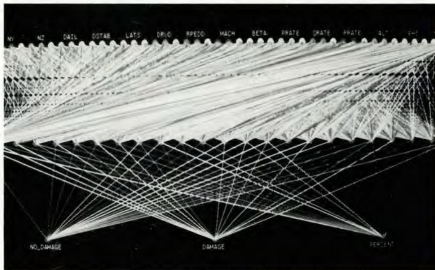
Figure 9. Neural Network Designed to Detect Wing Damage
