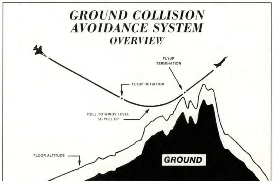
mishaps. Today, with the use of a digital terrain data base, their automatic All-Terrain Ground Collision Avoidance System (ATGCAS) is the technology almost eliminating this deadly and costly mishap category. Here's how it works.
