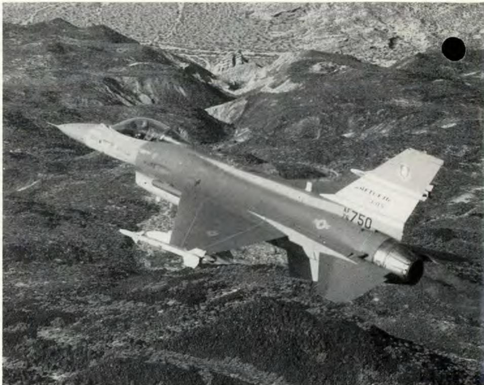
The difference between the AFTI/F-16 GCAS and other ongoing efforts is that it uses an automatic recovery. The system warns the pilot but if the pilot does not react, the system takes over and recovers the aircraft at the last possible moment.
