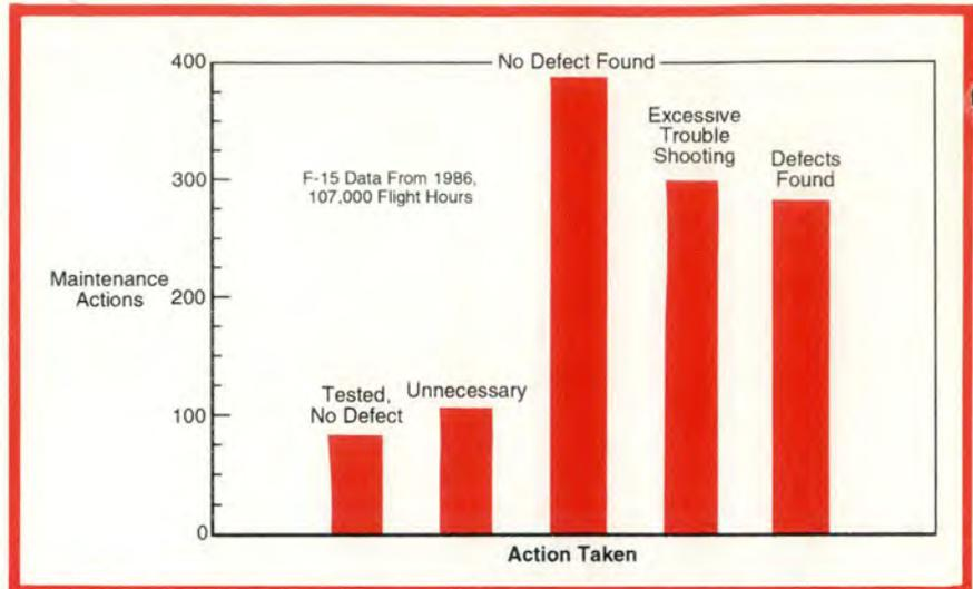
Figure 1. F-15 Maintenance Actions on Flight Control Subsystem Show Difficulty of Accurate Fault Diagnostics
