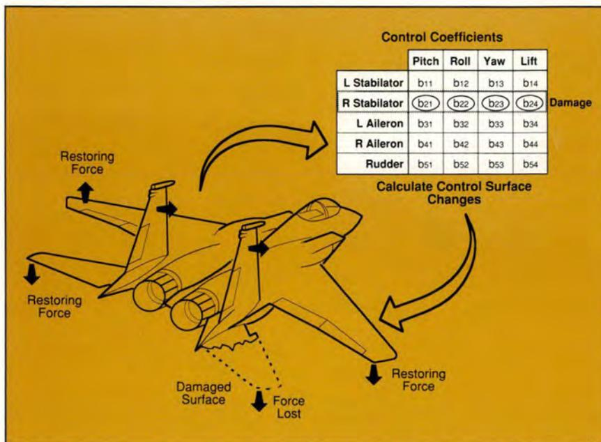
Figure 6. Reconfiguration Software Calculates Stabilizing Control Surface Commands
